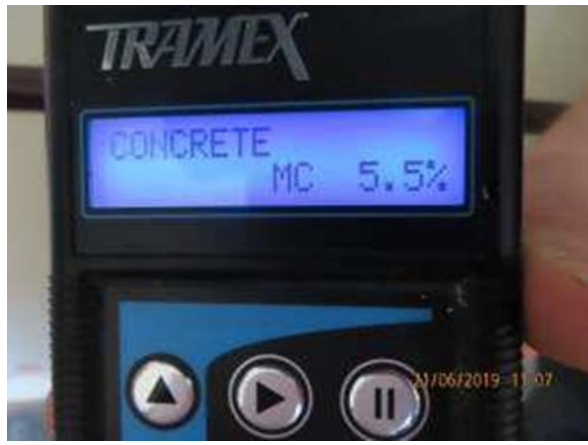
Concrete floor, wet and damp proof membrane, is suspected as faulty
