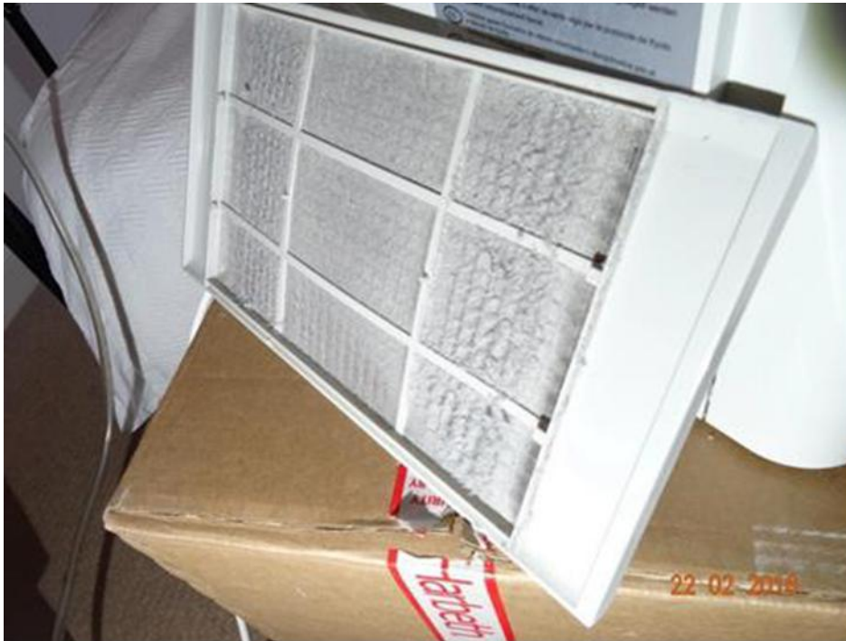
Mould growth on the internal filter of the dehumidifier
