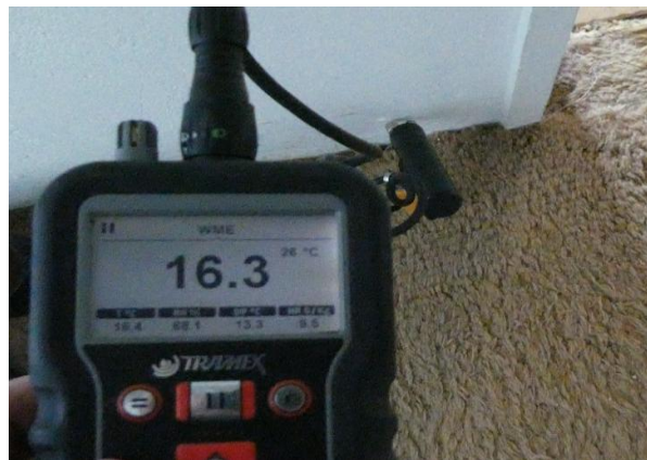
Comparison levels indicating lower moisture issue with likelihood of mould in cavity
