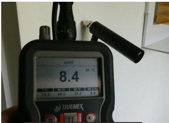
Comparison levels indicating lower moisture issue with likelihood of mould in cavity
